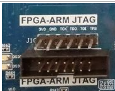
Figure 14.2 JTAG Interface Physical Picture
