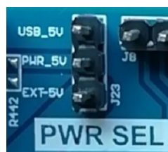
Figure 2.5 Power Supply Selection Jumpers
