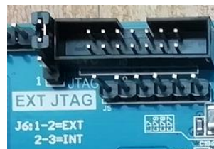
Figure 13.2 JTAG Interface Physical Picture
