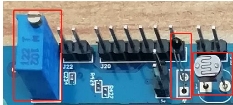
Figure 8.3 Thermistor, Photoresistor, and Potentiometer
