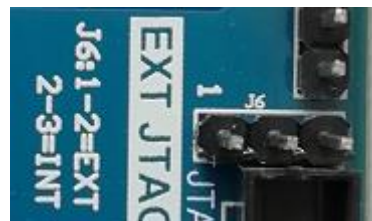
Figure 1.6 Program Download Selection Jumper J6
