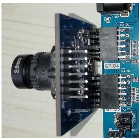
Figure 12.3 GPIO Interface with BD5640 Camera Daughter Board
