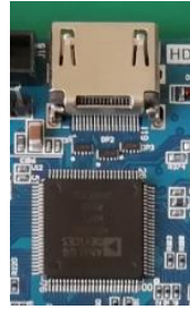
Figure 4.1 HDMI Interface and ADV7511 Chip
