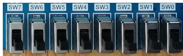
Figure 9.2 Toggle Switches Physical Picture
