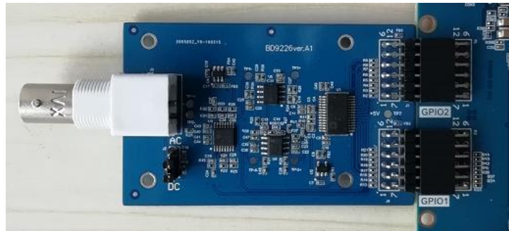
Figure 12.4 GPIO Interface with BD9226 High-speed AD Daughter Board
