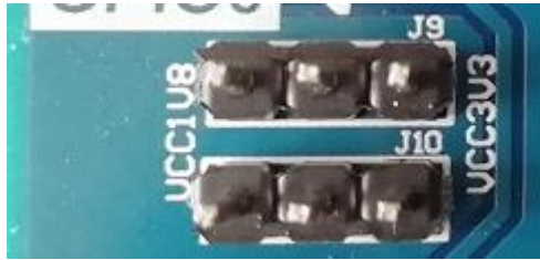
Figure 1.5 BANK Voltage Selection
