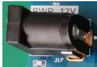
Figure 1.2 External Power Supply Interface
