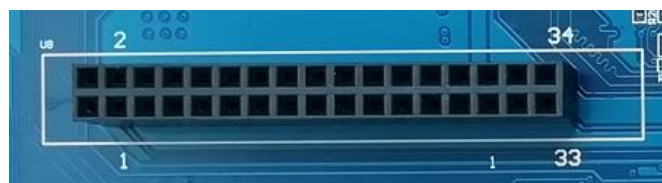
Figure 18.1 LCD Interface Physical Picture
