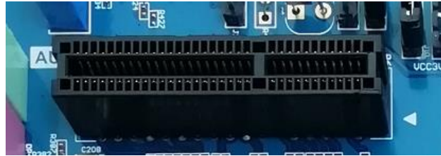
Figure 20.1 PCIe Interface Physical Picture
