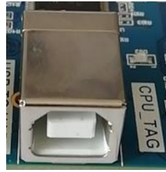
Figure 13.3 RISC-V Download Interface Physical Picture
