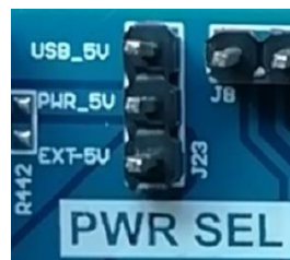
Figure 1.4 Power Selection Jumper J23
