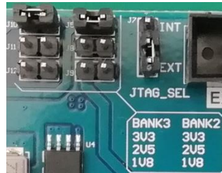
Figure 1.5 BANK Voltage Selection
