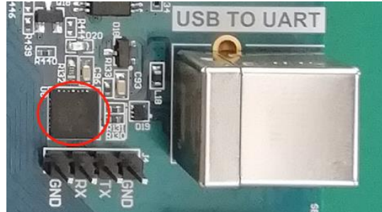
Figure 10.1 USB-B Interface and CP2102 Chip Physical Picture
